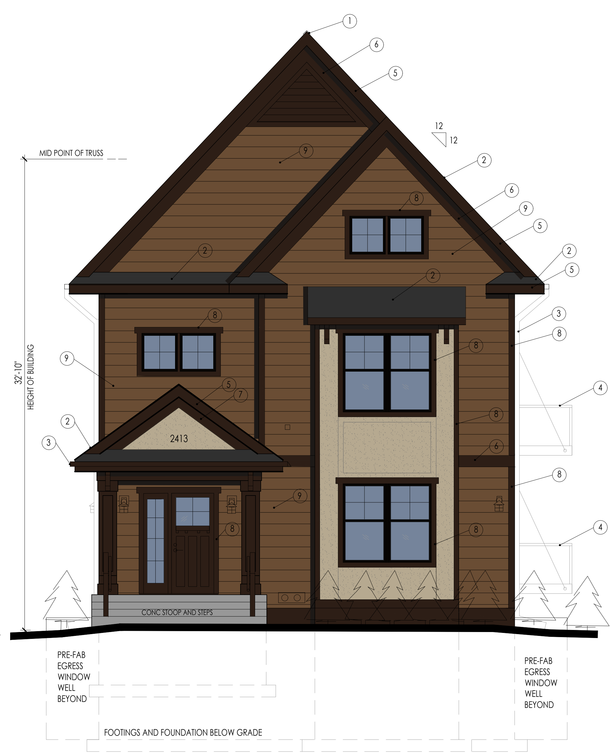
1 FRONT FACADE - WEST FACING SCALE: 1/4" = 1'-0"
