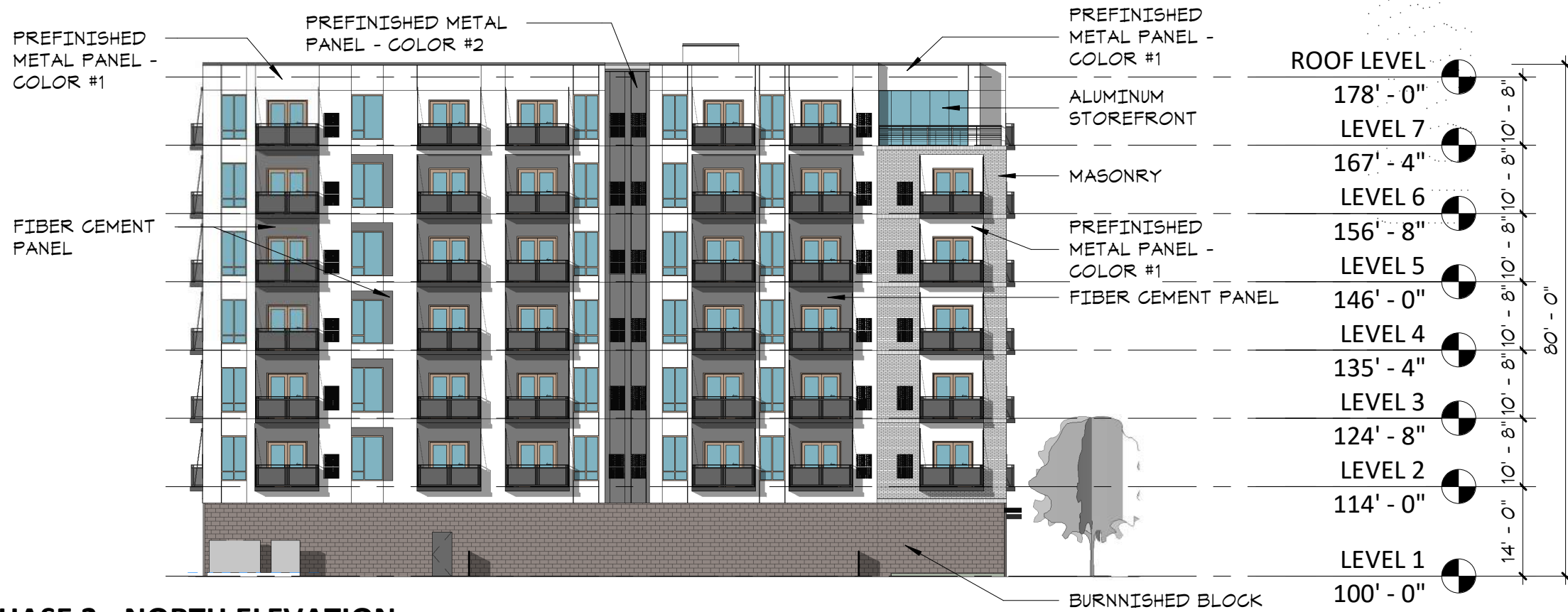
PHASE 3 - NORTH ELEVATION
